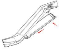
Push the top part of the battery into the frame, until you hear the battery lock into position, and turn the limiting stopper to keep the battery from dropping.
